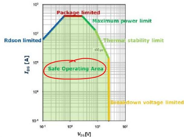
Fig. 4 Safe operating area diagram of a 25V Power MOSFET (BSC010NE2LS). The SOA is shown for 100 $\mu$ s pulse time and the limiting lines are indicated.
