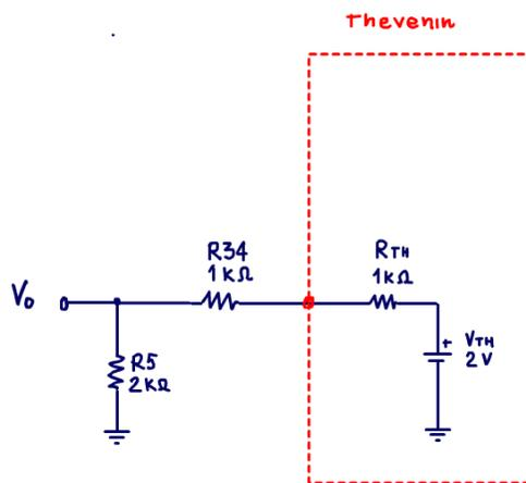
$$R_{34} + R_{TH} = 1k\Omega + 1k\Omega$$
