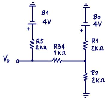
$$V_0 = V_{0B0} + V_{0B1}$$
