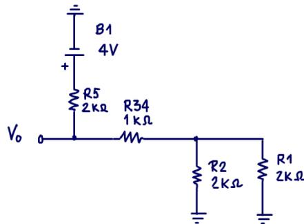
$$R_{12} = R_1 // R_2 = \frac{2k\Omega}{2} = 1k\Omega$$
