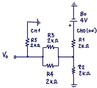
$$R_3 // R_4 = R_{34}$$
