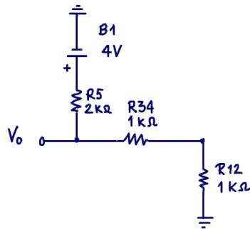
$$R_{1234} = 1\text{k}\Omega + 1\text{k}\Omega = 2\text{k}\Omega$$
